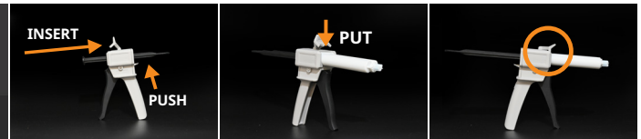
① Push the latch and insert the stick. ② Put the tube in. ③ Close the cover.
